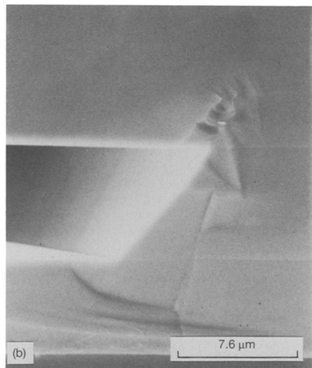
Figure 9 Scanning electron micrographs of (a) the right and (b) the left side of the fabricated silicon membrane.
